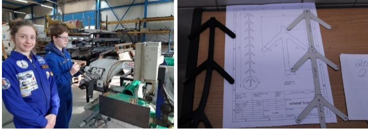
Production of the wheel segments by Cosma and Lennox, Water Jetting of the treads
